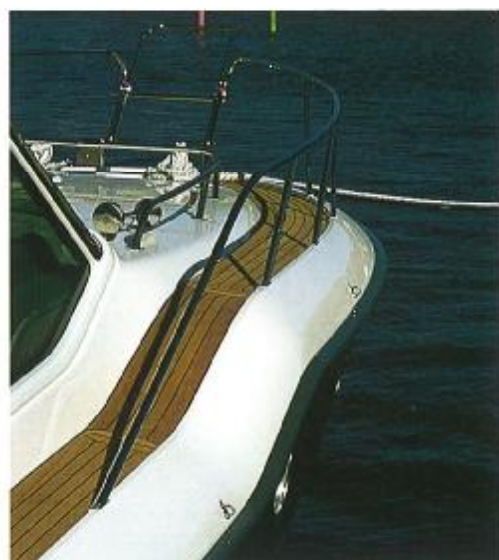
To ensure safety on the foredeck, the Storebro J32 can be fitted with a stainless-steel pulpit, including an integrated bathing ladder.
