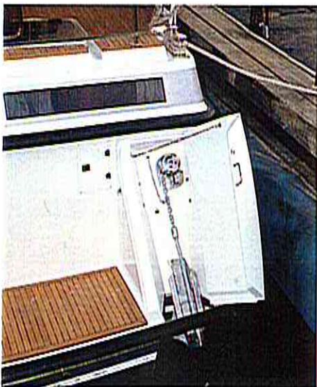
Neat stern anchor and windlass compartment
