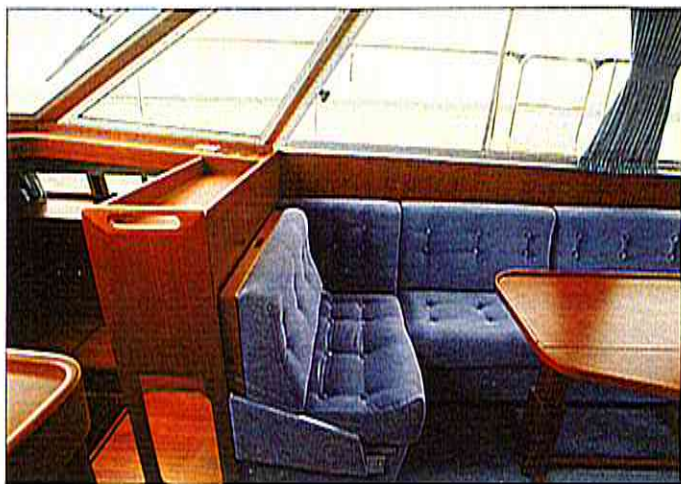
The arm of the saloon settee (left) flips over to form a forward-facing bench for two people (right).
