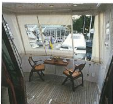
A cover is cleverly concealed underneath the flying bridge and can easily be unfolded to create a sheltered area of the afterdeck.
