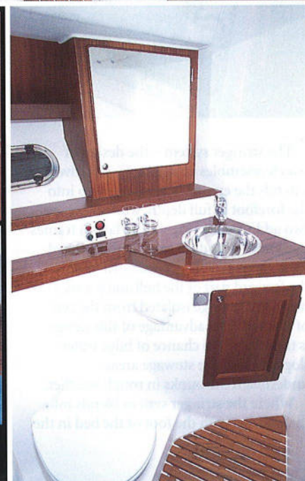
Top: roller doors can't spring open in rough weather. Above: deep fiddles double as handholds.
