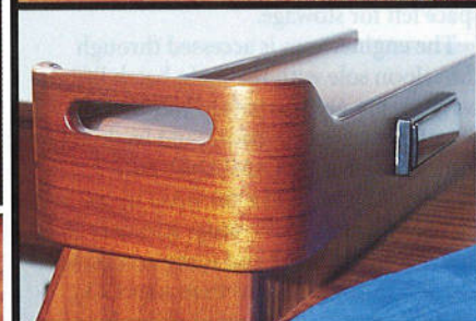
Top: roller doors can't spring open in rough weather. Above: deep fiddles double as handholds.
