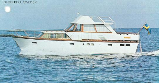
The Royal Cruiser 25 has hull and cabin top in glass reinforced plastic with superstructure and furnishing in mahogany — an advantage both with regard to safety and appearance as well as second-hand value. The cabin roof ceiling is entirely covered with insulating laminated vinyl as is the hull interior. The floor of the cabin is covered with close
