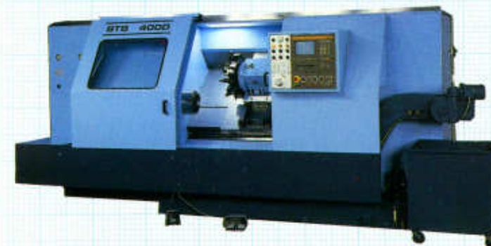
STOREBRO STB 4000 working area between centres \varnothing 325x950 DC-drive 44 kW, spindle speeds up to 4000 r/min
