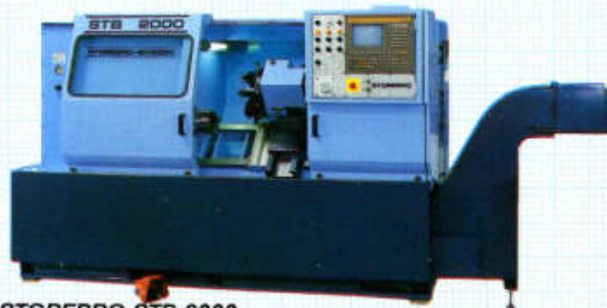
STOREBRO STB 2000 working area between centres \varnothing 240x675 mm DC-drive 11 or 22 kW, spindle speeds up to 6000 r/min
