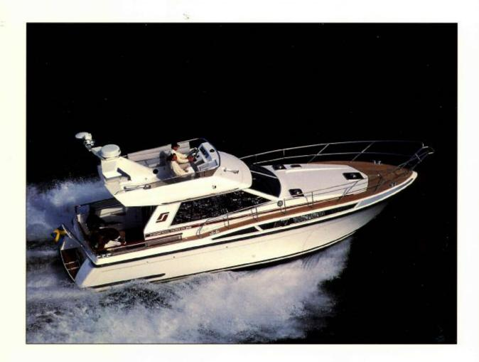
The Storebro Royal Cruiser 380 Biscay is the first of a new generation of boats from Storebro. It features a completely new hull design, with a deeper V-shape and propeller tunnels, to cope with more powerful engines and higher speeds, while retaining the same steady performance. The reverse sheer stern and gull-wing mast on the flying bridge are other noticeable characteristics of these new models.
