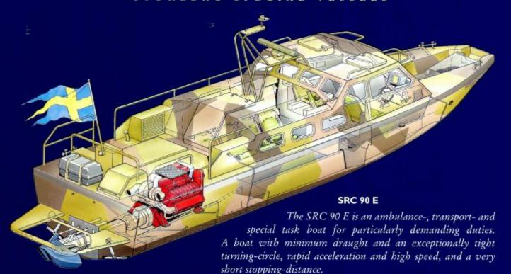
The hull and superstructure are made from a carbonfibre reinforced vinylester sandwich. The keel and bottom
