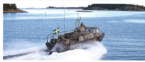
lions, the job was awarded to Storebro. The new vessel, the SRC 90 E, has an advanced design featuring several innovations, including a carbon fibre reinforced hull and water jet propulsion. This extremely fast, easily manoeuvred boat can operate in very shallow waters and can even be run up onto the beach, if required.
