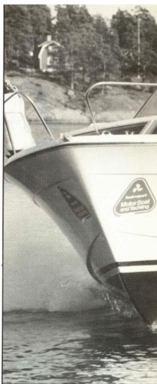
Above, at speed in the smooth, inter-island waters off Vastervik. Right, in the Baltic proper, the knuckle keeps spray low
