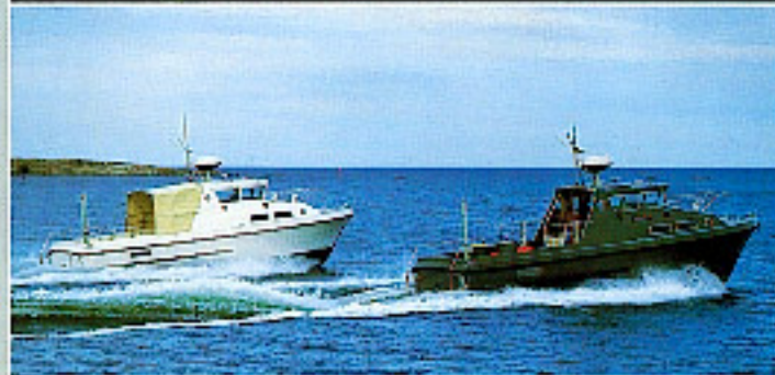
STOREBRO 34 WORKBOAT L.o.a. 10.35 m, displ. approx 6 tons, speed up to 25 knots
