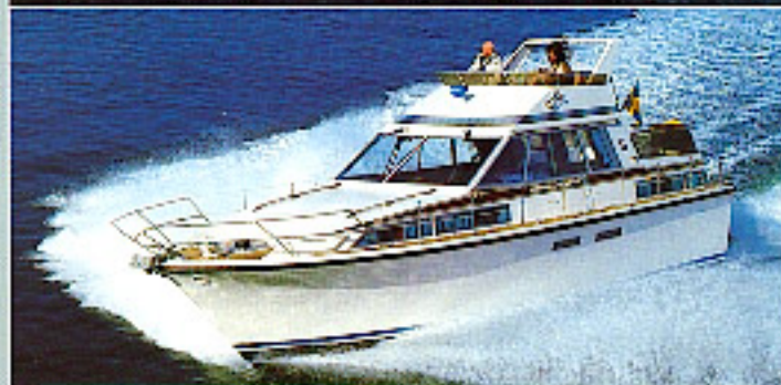
STOREBRO ROYAL CRUISER 40 BALTIC L.o.a. 12.09 m, displ. approx 11 tons, speed up to 25 knots
