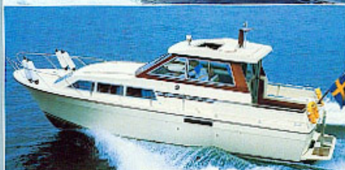
STOREBRO ROYAL CRUISER 31 BISCAY L.o.a. 9.30 m, displ. 4.5 - 5.5 tons, speed up to 30 knots
