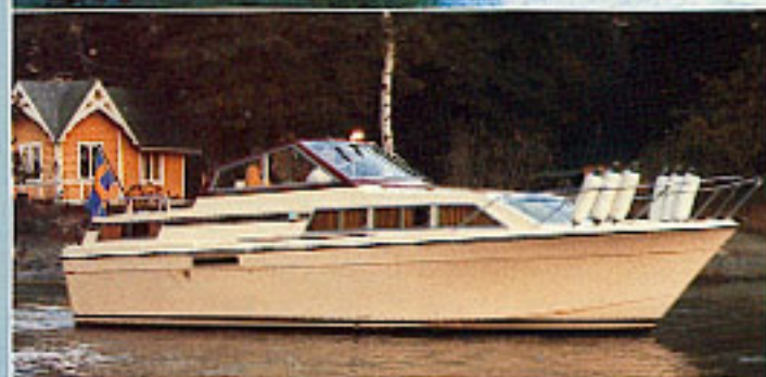
STOREBRO ROYAL CRUISER 31 BALTIC L.o.a. 9.30 m, displ. 4.5 - 5.5 tons, speed up to 30 knots
