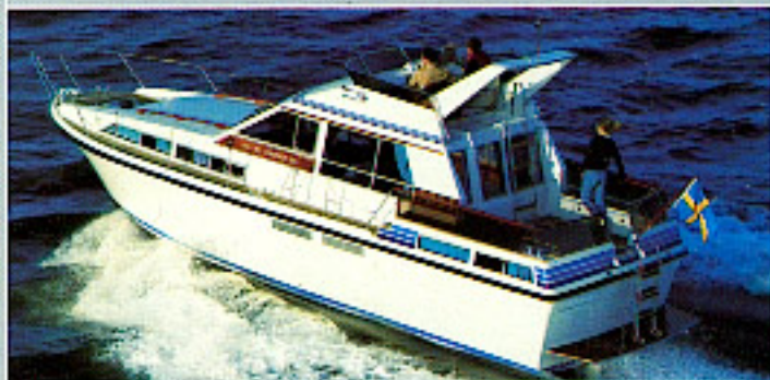
STOREBRO ROYAL CRUISER 36 BALTIC L.o.a. 11.00 m, displ. approx 9 tons, speed up to 24 knots
