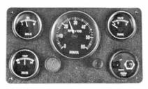
Instrument panel, which is extra equipment, is provided with key switch, rev counter, temperature gauge, oil pressure gauge, Voltmeter and switch for instrument lighting.
