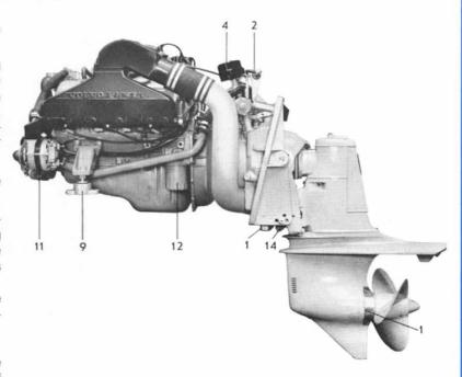
Reversing pawl (14) of patented design permits the drive to kick up when striking underwater objects. Yet holding the drive in downward position when going in reverse or pulling back the throttle rapidly in forward motion.
