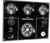
The instrument panel is provided with a key switch, rev counter, temperature gauge, oil pressure gauge and voltmeter, warning lamp for connection of glow plugs, reostated switch for instrument panel light. Cable harness, 7 m (23 ft.) in length, with plug-in contact already fitted, for connection to engine and instrument. Control lamp and switch for drive lift and 7 m (23 ft.) electric cable harness with plug-in contact are also supplied.
