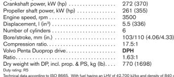
Technical data according to ISO 8665. With fuel having an LHV of 42,700 kJ/kg and density of 840 g/liter at 15°C (60°F). Merchant fuel may differ from this specification which will influence engine power output and fuel consumption. The engine complies with IMO NOx and the comprehensive emission requirements US EPA Tier 2 and EU RCD.
