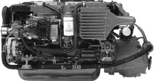
The hydraulically shifted reverse gear, HS1E, is developed to increase the standard of comfort in terms of quiet running, greater reliability and enhanced efficiency.
