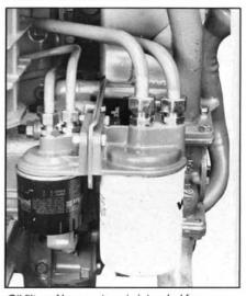
Oil filter of bypass type is intended for engines with long operating periods and can, subject to regular oil sampling, extend the oil change intervals. Mounted on front of engine for easy replacement.
