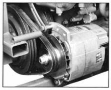
There is a choice of four alternators for the TAMD71A: 12 V/50 A, 24 V/55 A, and extra alternators of 12 V/130 A and 24 V/100 A output.
