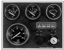
Instrument panel with clear and easily-read ISO-symbols for temperature, oil pressure and charging. Double glazing of instruments prevents condensation. Key-operated switch with starting and stopping functions and built-in starter motor protection.
