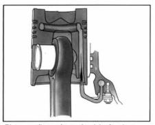
Piston cooling reduces the risk of carbon deposits. For maximum resistance to wear, the top piston ring is chromed and lies in a special ring carrier of cast iron.
