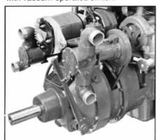
Front-mounted 10" power take-off. Disengageable. An extra 24 V/100 A alternator is fitted as well as a bilge pump and a flushing pump.
