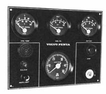
The instrument panel is provided with a key switch, rev counter, temperature gauge, oil pressure gauge and voltmeter, warning lamp for connection of glow plugs, reostated switch for instrument panel light. Cable harness, 7 m (23 ft.) in length, with plug-in contact already fitted, for connection to engine and instrument.
